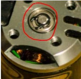
Firstly, disassemble the motor by removing the c-clip on that back of the motor and separate the motor into two pieces. The stator along with any other loose parts should be set aside and placed into a small plastic tub for safe keeping.
