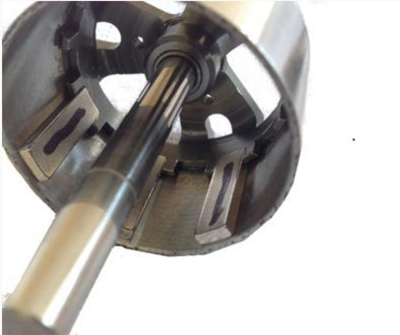
Place the rotor back onto the motor and spin to make sure that it spins freely. If the rotor does not spin freely you should remove the rotor and grind off any of the offending CA and baking soda that could be touching the stator. Once the rotor spins freely you can reassemble the motor and take it up for a spin.
