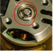
Firstly, disassemble the motor by removing the c-clip on that back of the motor and separate the motor into two pieces. The stator along with any other lose parts should be set aside and placed into a small plastic tub for safe keeping.
