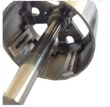
Place the rotor back onto the motor and spin to make sure that it spins freely. If the rotor does not spin freely you should remove the rotor and grind off any of the offending CA and baking soda that could be touching the stator. Once the rotor spins freely you can reassemble the motor and take it up for a spin.
